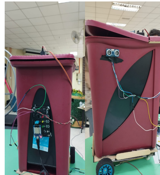
Smart trash can: monitor the volume of trash, automatic open and close system, and operate the wheel by phone
